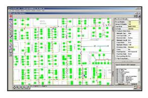
The GDI includes a wide variety of tools for modifying the pipe, node, and customer model features including routines for adding, deleting and moving features - and the ability to undo accidental changes and deletions. Three independent display panels support various zoom
